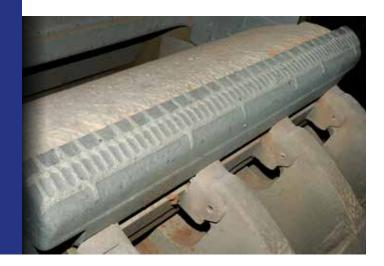
**Recyx®** has a carbon content allowing it to reach a toughness of >100 J/cm² along with an increase of its lifetime. Whilst most competitors tend to increase the carbon content, which reduces the toughness below 50 J/cm² and increases the risk of breakage as a consequence.
