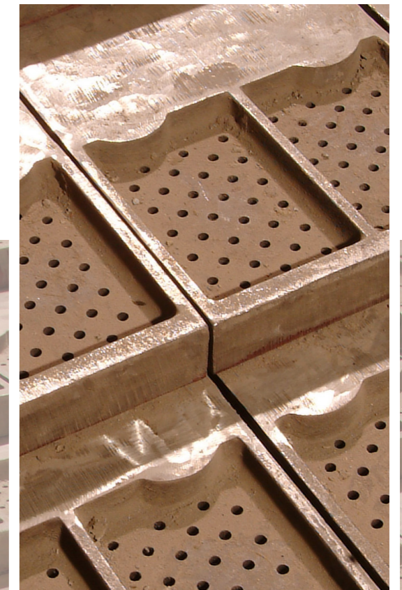
Pocket grates installed in a 4600 tpd cooler in Belgium
